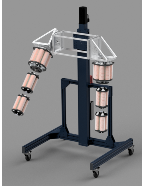
Figure 1: Rendering of preliminary robot torso design. This will be used for hardware testing of whole-arm manipulation tasks in this thesis. For scale, the entire structure is about 1.8 meters tall.
