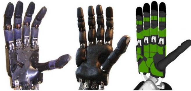
Fig. 2. Shadow Dexterous Hand (left) that has been covered with a tactile skin [51] (middle) in order to provide tactile information at several locations (highlighted green regions on the right rendering).
